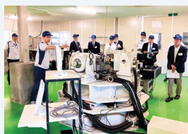
▲Demonstration of the 3-axis 6-degree-of-freedom vibration table
