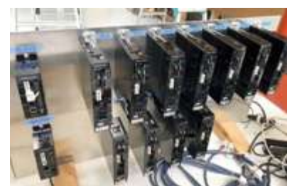
▲Replacement of Servo Motors, Drivers, and Controllers
