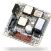
MEMS IMU Attitude angle accuracy 0.1°
